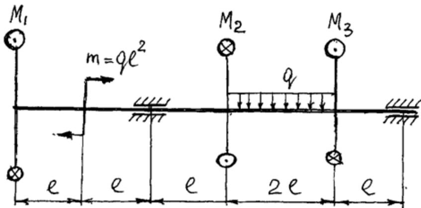
$$\begin{aligned} M_1 &= 2qe^2 \\ M_3 &= 2qe^2 \\ e &= 1 \text{ м} \\ q &= 10 \frac{\text{kH}}{\text{m}} \end{aligned}$$
